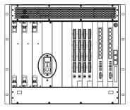
Use the rear panel power switch to switch off the MPS power.
